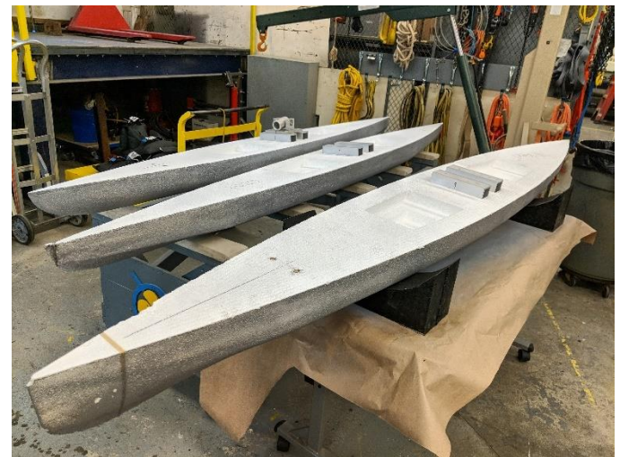
Figure 1. Three scale model hull designs were resistance tested in the hydrodynamics lab. From farthest to nearest: KEPLER -New L/B, KEPLER , and V-keel Hull.
