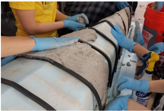
Figure 4. Foam tape used to maintain uniform thickness in each layer of TERRA
