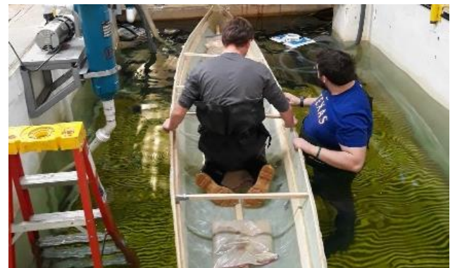
Figure 2. Hull design leads test practice canoe for leaks
