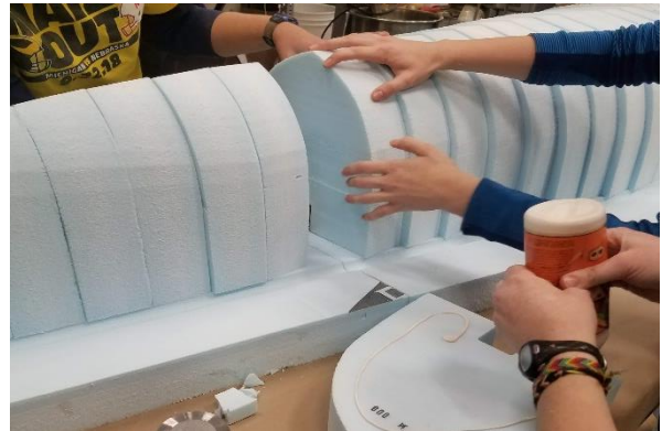
Figure 3. Assembly of form used to cast TERRA
