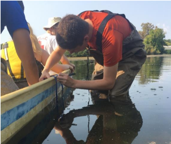
Figure 3. Hull testing of VALIANT to determine accurate waterlines and load cases.
