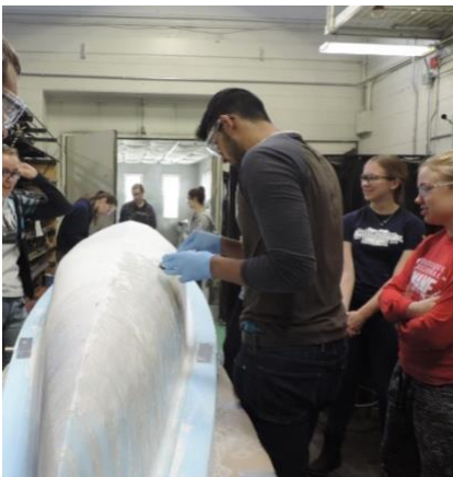
Figure 8. Applying release coating to the exterior of the mold.
