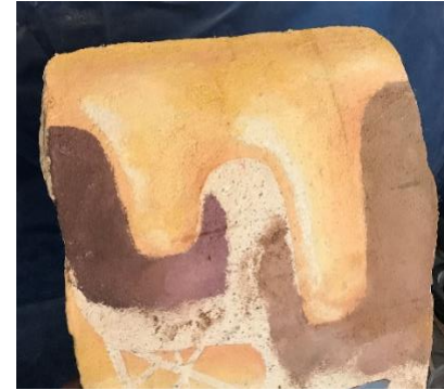
Figure 7. Aesthetic testing using various pigment proportions in the finishing mix.
