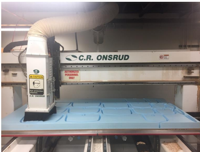
Figure 12: CNC Router Cutting Sections from Foam Sheets
