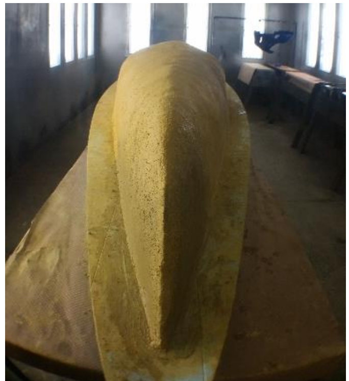
Figure 11: Pigmented Concrete Canoe
