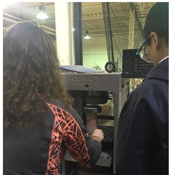
Figure 10: Compression testing of concrete cylinders
