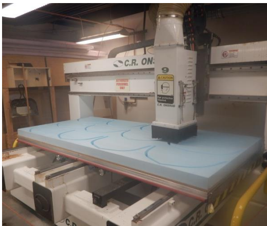
Figure 12: CNC router cutting sections from foam sheets
