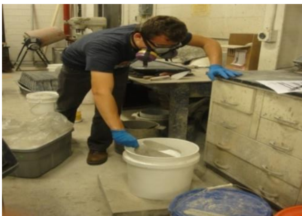
Figure 6: Measuring aggregates and cementitious materials during mixing
