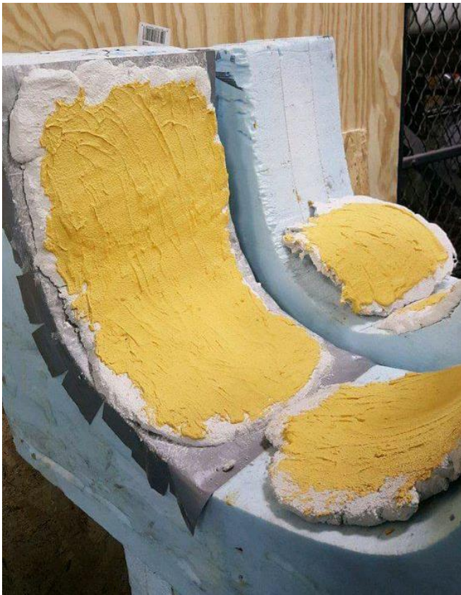
Figure 11: Testing release agents and pigments
