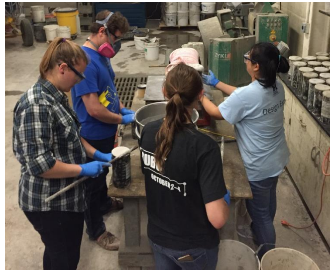
Figure 9: Packing cylinders for compression and tensile testing
