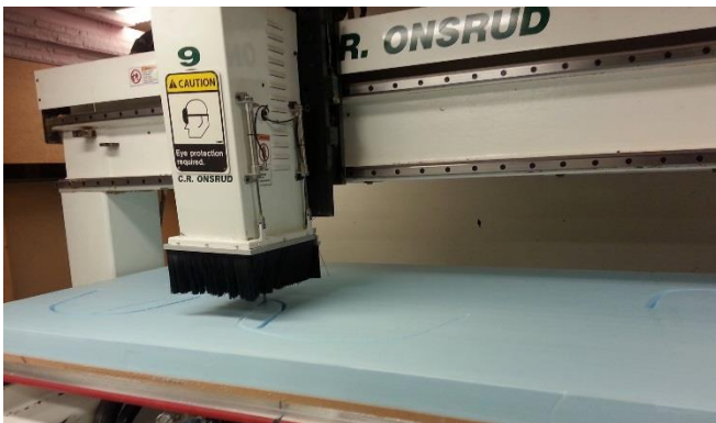
Figure 10: CNC router cutting sections from foam sheets
