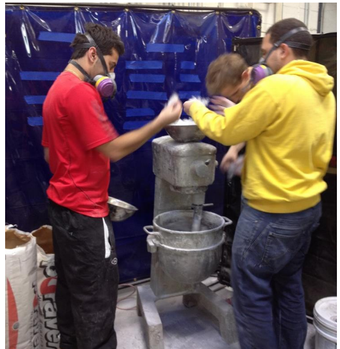
Figure 6: Testing increased cementitious to aggregate ratio
