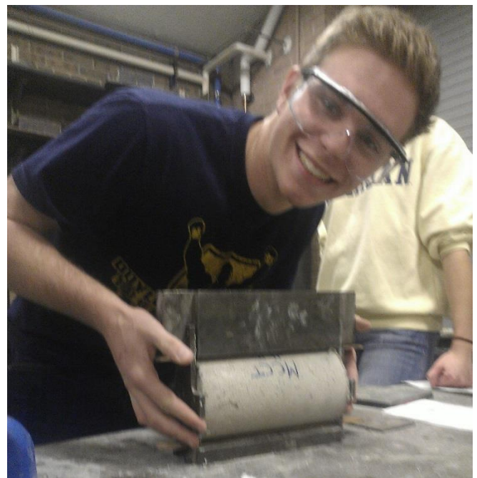
Figure 8: Tensile testing of concrete cylinders
