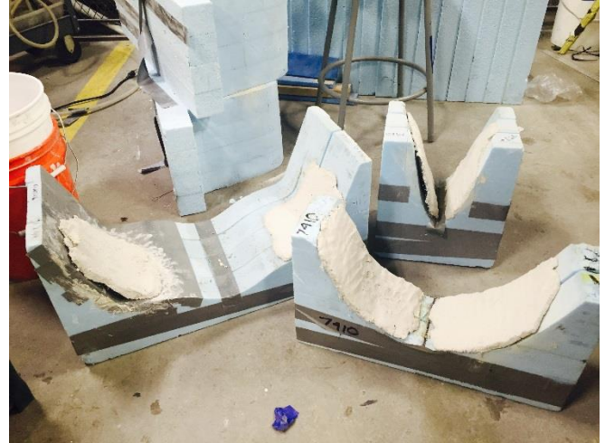
Figure 9: Testing release methods using female mold sections
