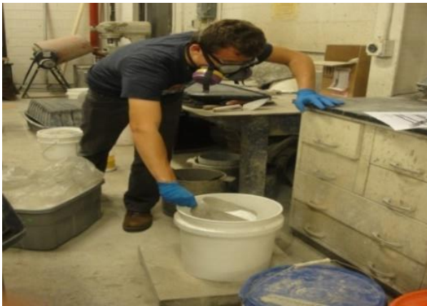
Figure 5: Measuring aggregates and cementitious materials during mixing
