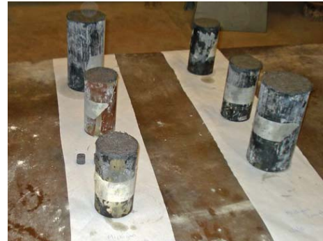
Figure 3: Two Test Batches. Because all five concrete batches proved to be equally workable and had approximately equivalent densities, strength was the deciding factor for the final mix design.
