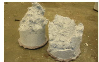
Figure 10: Compression Test cylindrical specimen.
