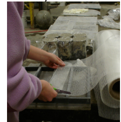
Figure 11: Plate test Preparation w/ mesh.
