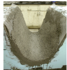
Figure 12: Canoe Test Section w/ mesh layer
