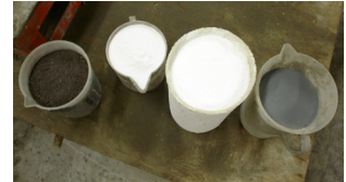
Figure 7: Concrete materials. (left to right) Haydite, S-38, EPS, Cementitious materials
